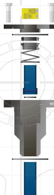
COMPONENT MECHANICAL SEAL ASSEMBLY
