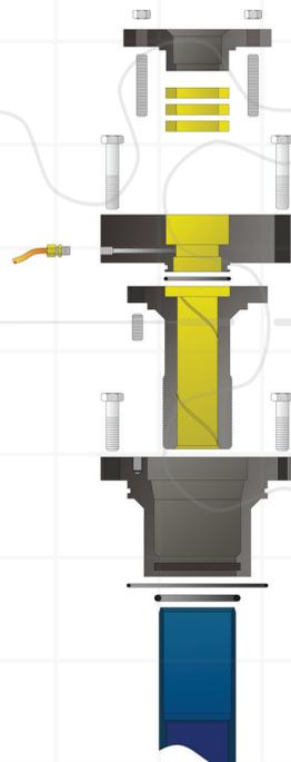
WATER FLUSH PACKING GLAND TENSION NUT ASSEMBLY
