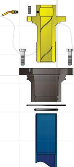
OIL LUBE TENSION NUT ASSEMBLY
